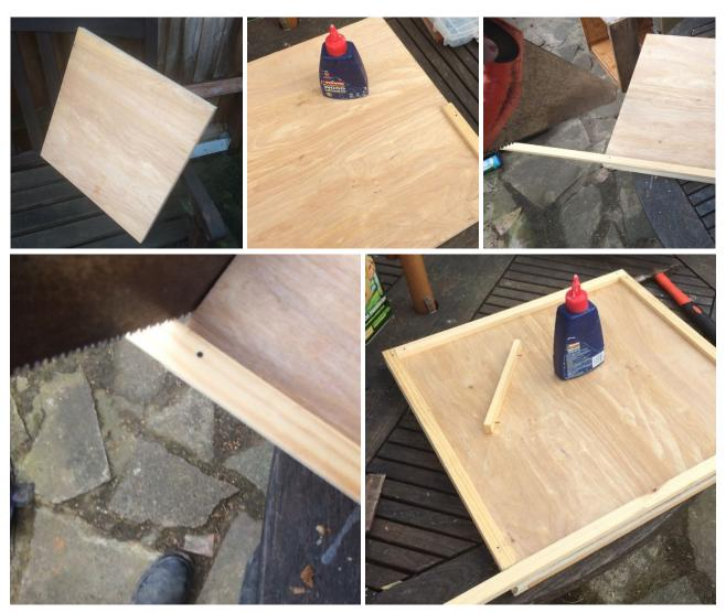
Making a crownboard. From the top left: a plain 46cm plywood board; temporally nailing the strip of to one edge in the corner; trimming the strip so it's flush with the edge; repeat for side 2; repeat for side 3; remove the temporary strip and complete slide 4.
