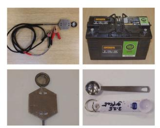
(Top left) Varrox® sublimator, 12v and 150 W. (Lower left) Close-up of the heated cup at the end of the sublimator into which the oxalic acid crystals are placed. (Top right) Leadacid battery, 115 Ah, capable of powering the sublimator for approximately seven hours. (Lower right) Half-teaspoon measures are cheap to buy and are a convenient way of dispensing oxalic acid crystals for sublimation as half a teaspoon, 2.5ml, of oxalic acid crystals is almost exactly 2.25g.
