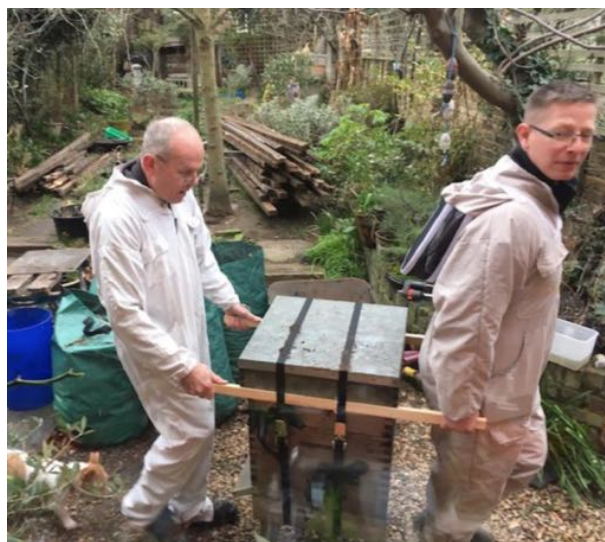
Testing the prototype hive carrier promised in the risk assessment. We rejected a proprietary one on the grounds of poor design and poor welding quality. The handles shown here cost considerably less than £55!
